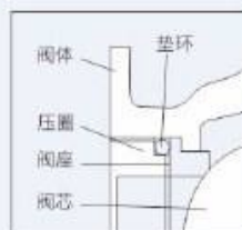
图1 软密封结构局部图 Figure 1 Soft seal structural diagram
