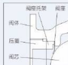
图2 钢片式金属硬密封结构局部图 Figure 2 Steel sheet type metal hard seal structural diagram
